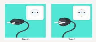
Plug type C has two round pins and type F has two round pins with two earth clips on the side.
